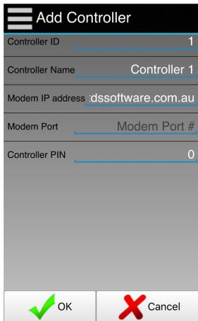
The Controller Add and Edit screen allows the user to configure additional controllers. When adding a controller, default values are used. The Modem Port is a unique number provided with each Remote Access Gateway. The Modem Port number is located on a tag connected to the antenna connector. It is also located on the bottom face of the gateway enclosure, and can also be found through the communication module setup screen on the controller.
