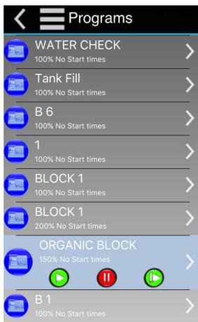
The Programs List shows the list of 32 programs in the controller and the status of each program. Selecting a program displays command buttons appropriate for the current program status. These command buttons allow programs to be started, stopped, paused, resumed or skipped. Note that when a button is pressed, the command is sent to the controller and it may take a short period of time for the command to be acted on by the controller and the new status to be reported and displayed.
